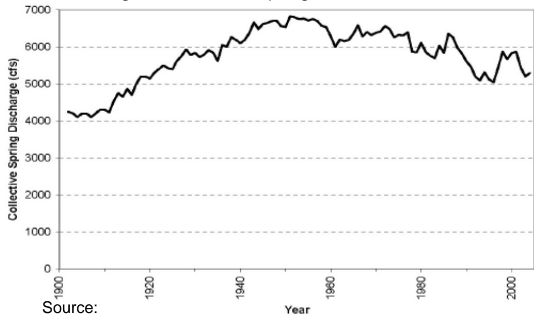
Discharge at Thousand Springs reach of the Snake River
